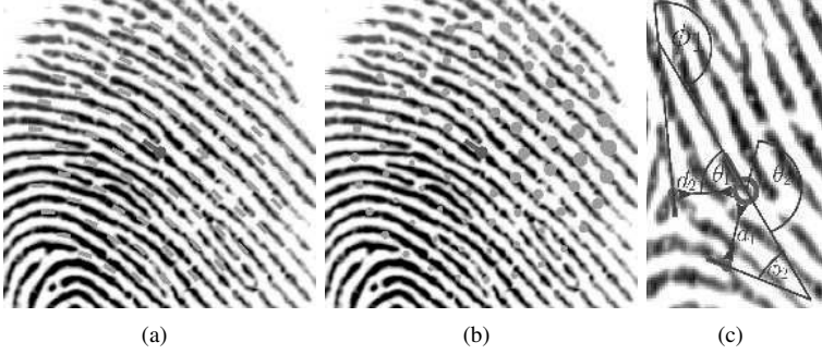
Figure 1: Minutia orientation descriptor (a) and minutia frequency descriptor (b) consist of local orientation and ridge frequency estimations, respectively, sampled on 76 coordinates equidistantly spaced around the reference minutia. A local minutia local structure (c) is a six-length vector (d_1, d_2, \theta_1, \theta_2, \phi_1, \phi_2) encoding the constellation of a the reference minutia and its two spatially closest neighboring minutiae.
