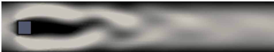
Fig. 1: Representation of the Kármán vortex street: The fluid flows from the left side into a channel and flows around an object on the left side to the right side of the channel. Typical, counter-rotating vortices are created behind the object.
