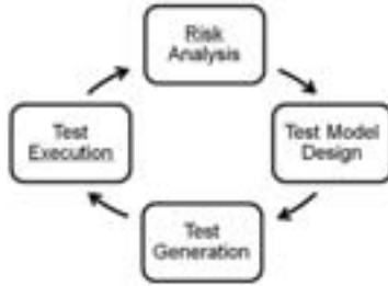
Figure 2: Overview of the Risk-Based Model-Based Security Testing Process
