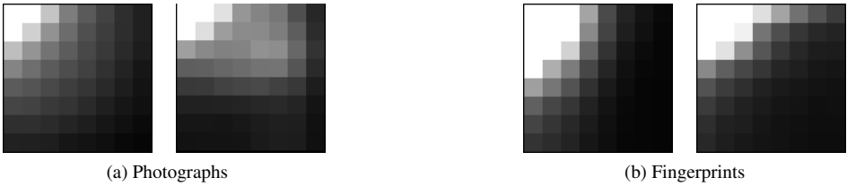
Figure 1: Average DCT coefficients of generic and fingerprint images (lighter areas indicate higher values)
