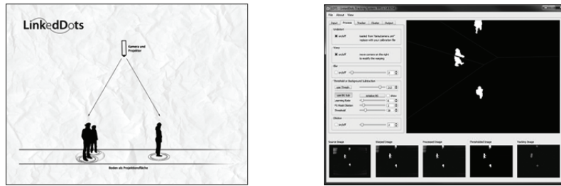
Figure 2: LinkedDots System. Camera and Projector mounted above (left). GUI of the tracking (right).
