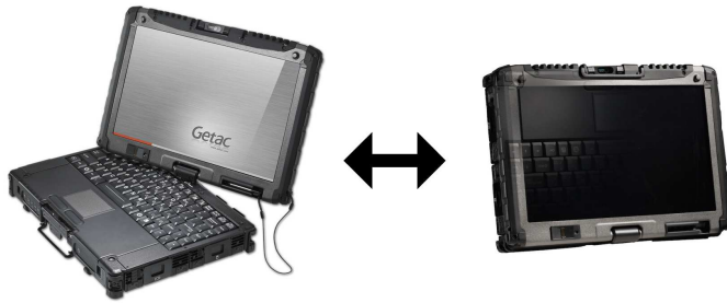
Figure 3: The Getac V200 is a convertible tablet PC with a full keyboard. The tablet mode can be seen on the right.
