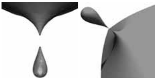
Figure 4: Left: a robust meshing algorithm employing interval arithmetic and dual marching cubes fails to determine the correct connectivity of a surface, likely due to insufficiently fine geometric sampling [PLLdF06]. Right: ray tracing using a similar interval arithmetic technique can also experience difficulty sampling thin features, but samples in a view-dependent fashion and thus better recovers features for closer views [KHH + 06].
