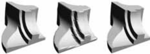
Figure 3: Piecewise-smooth partition-of-unity implicit reconstruction of raw point data, reconstructed with high polygonization, coarse polygonization, and sphere traced (e.g. Hart [Har96]). From Ohtake et al. [OBA + 03].
