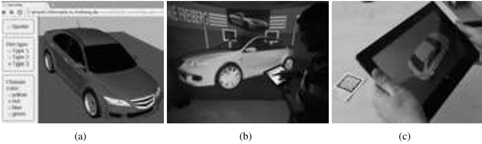
Figure 4: (a) 3D application in Web Browser; (b) CAVE-version of the application; (c) Prototype of an AR port of the application.
