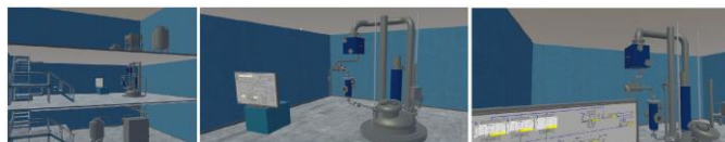
Fig. 1: The VR Prototype would span three levels (left) of a large building in real life, which would be costly to realize as a pure training environment. The main area (middle) hosts the reactor and the control panel (right, enlarged for visibility reasons)
