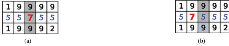
Figure 3: Excerpts of a DEM where two squares overlap in the gray-shaded boundary cells. Numbers in each cell of the DEMs correspond to the elevation. In both examples, the D8e algorithm extends the neighborhood of the cell with altitude 7 and precalculates the flow directions of all cells with altitude 5.
