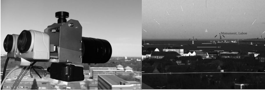
Figure 1: Hardware overview of the ARBinocular. Left: Device with augmentation camera (right), fisheye heading sensor (top), accelerometer (bottom) and binocular display (left). Right: Image of AR Device, the original with overlays of nautical data as seen by the user.
