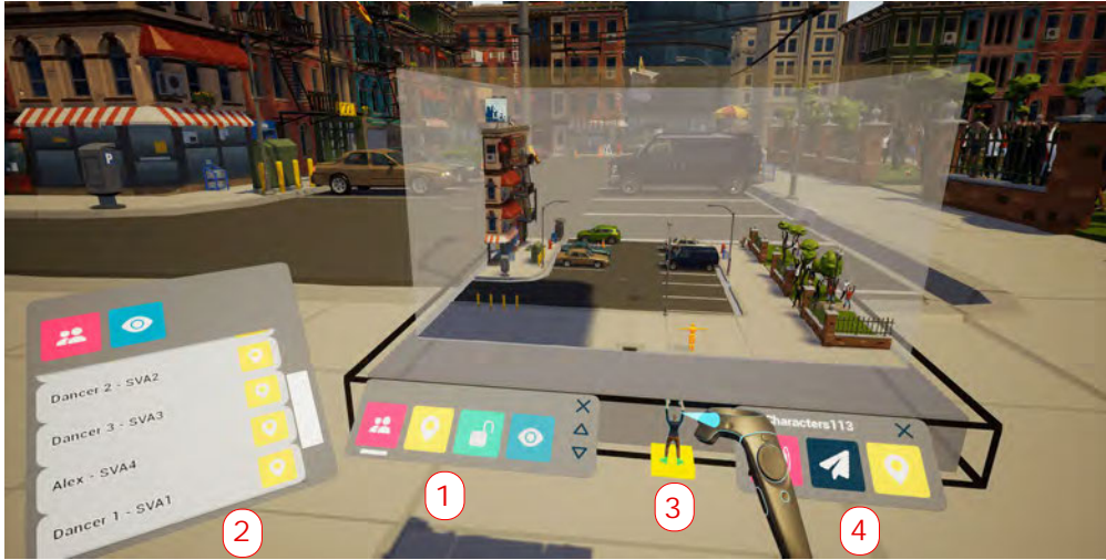
Figure 1: Our WiM setup with four interface elements located on the WiM’s exterior: a WiM options panel (1) for general control, an overview panel (2) offering a list of all VAs and an individual localization option, and a temporary storage box (3) and an agent panel (4) for VA orchestration.
