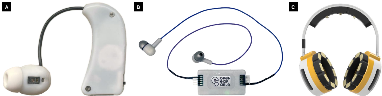
Figure 1: (A) OpenEarable, an in-ear sensing earable with a PPG, optical temperature, pressure, and IMU sensor as well as 2 ultrasound capable microphones; (B) OpenEarable ExG, a platform for sensing in-ear-based biopotentials; (C) Open ExG Headphones to measure biopotentials around the ears based on OpenBCI [7].
