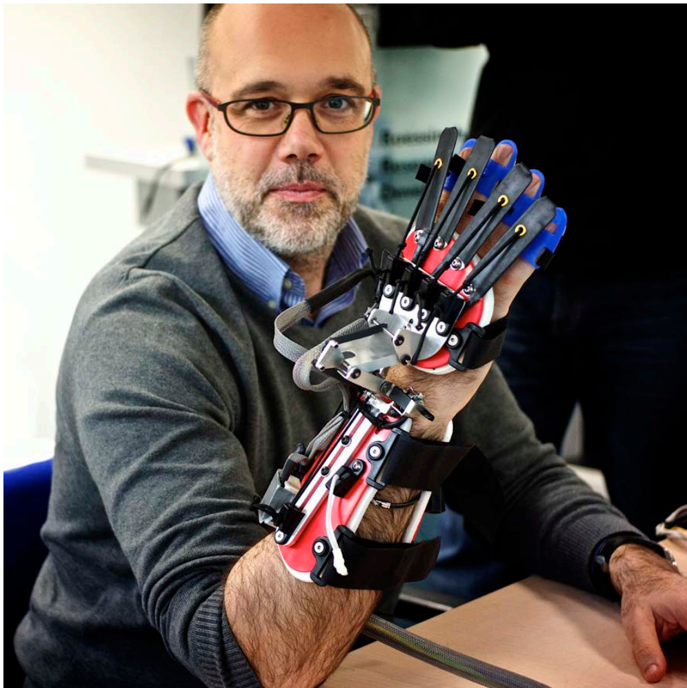
Figure 1: First prototype of robotic glove, worn by a healthy subject
