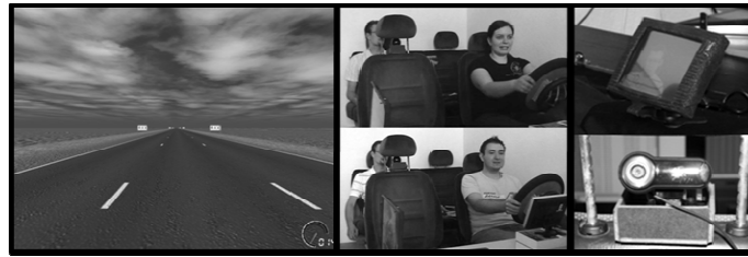
Figure 2: LCT screenshot (left), Driver with no video system (middle-top), Driver using video system (middle-bottom), Monitor display (right-top), Rear-seat webcam (right-bottom)
