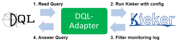
Figure 1: Query answering process using Kieker APM and Kieker4DQL adapter
