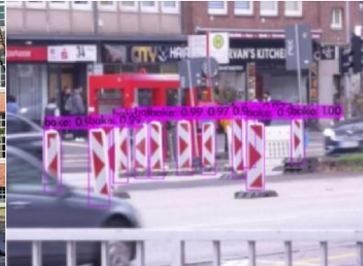
Fig. 5: Detector for construction-site beacons [GWH23]
