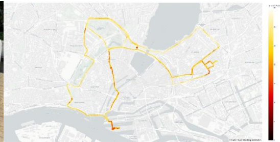
Fig. 9: GNSS-performance along the test track for automated and connected driving (TAVF) [WE23]
