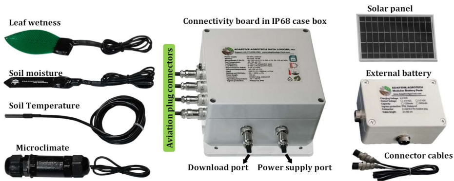
Fig. 3: The hybrid data logger with modular solar charged external battery and plug-and-sense probes used for validation of the wireless sensor
