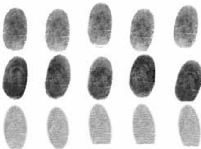
Figure 8: Samples of fingerprint data from a forefinger used in the evaluation. The first row contains LScan samples with 7N contact pressure. The second row contains LScan samples with 30N contact pressure at simultaneous lateral distortions (left, right, up, down, rotational). The third row contains contactless fingerprint captures.
