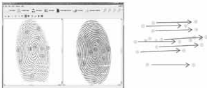
Figure 7: (a) Labelling software to annotate corresponding points in TF3D finger images (left fingerprint image) and contact-based scanner images (right fingerprint image). (b) Resulting corresponding points.
