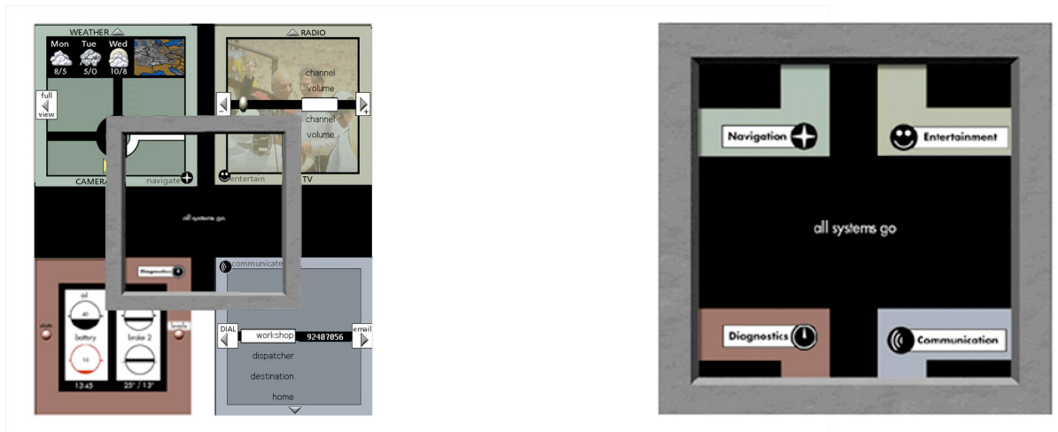
Figure 1: Conceptual model (left) and the resulting display content (right) in their stand-by state. The four-segment panel is in its center position.
