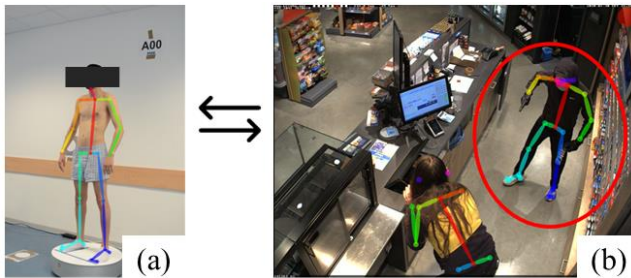
Fig. 5 Comparison of the digital skeleton of a known person, generated by "OpenPose", during an extended measurement service (a) with a digital skeleton of an unknown person, captured by a surveillance camera of a gas station (b).
