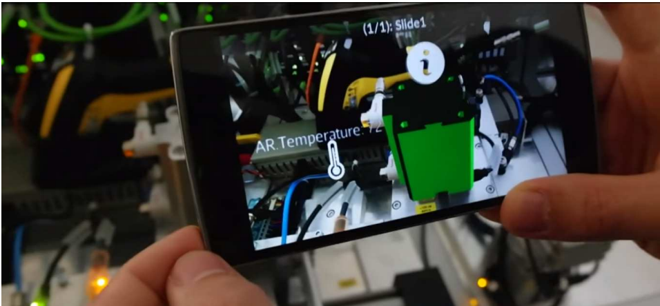
Fig. 5: Case study showcasing real-time information communicated via OPC UA in an AR scenario.
