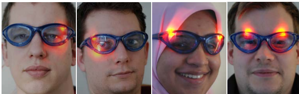
Figure 4: Two typical examples for encoding the directions left and right are shown in the two leftmost images. Every participant preferred to exclusively switch on LEDs on the according side of the glasses. Two almost equal-looking representations of behind and ahead are shown in the two rightmost images. Every participant switched on at least one LED per side to encode these two directions.
