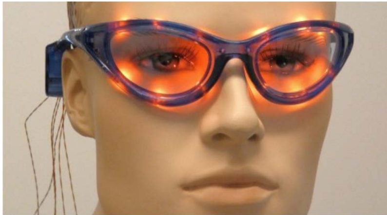
Figure 1: A mannequin with AmbiGlasses. The glasses consist of 12 LEDs that can be switched on or off separately.
