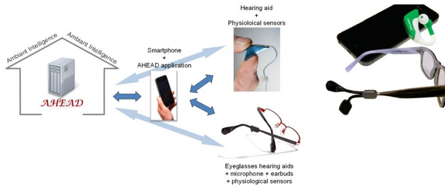
Figure 1: Architecture (left) and prototype (right) of the technological approach
