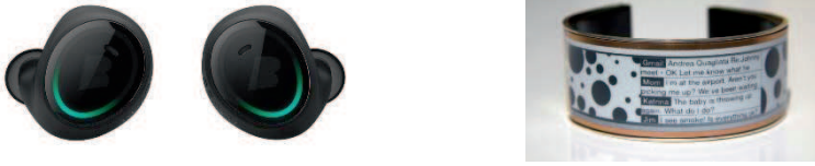
Fig. 2: (a) „Earable“ seamless, wireless smart earphone / (b) Eyecatcher fashion e-ink bracelet
