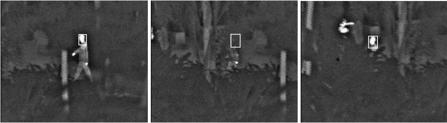
Figure 3: A tracker working with the IR video: frames 1570, 1625 and 1670. The object is lost after the full occlusion, but recovered after that.
