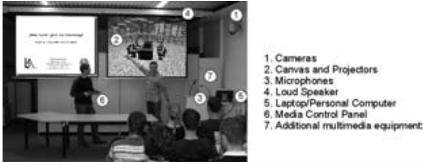
Figure 2: Scenario and technical equipment for computer-aided face-to-face learning in a media lab
