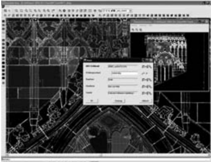
Figure 1: Digital map with recorded facade damages, St. Stephan, Passau
