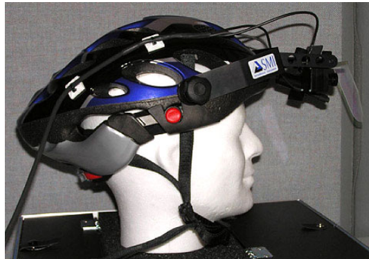
Figure 2: The mobile eye-tracker
