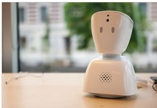
Figure 1: The telepresence robot AV1 from “No Isolation” is used in many schools to enable ill children to participate in classes remotely.
