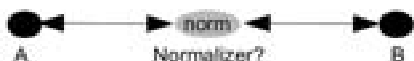
Figure 1: Communication between two hosts A and B. Neither A nor B know about the existence of a normalizer (and its configuration) between them a priori.
